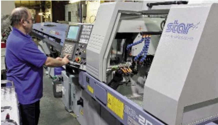
DKW Engineering has decommissioned over 60 cam autos since 1997, replacing them with seven Star sliding-head machines. The company has retained oil industry work
