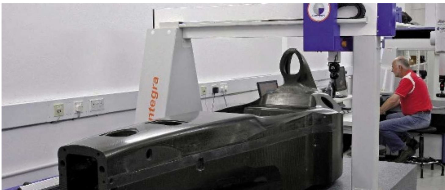
Super Aguri F1 is using a Metris LK CMM with 2,500 by 1,000 by 800 mm envelope to measure complete race car chassis
