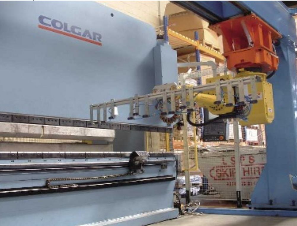
A £400,000 automated press brake installation based around Colgar machine, Starmatik material handling and Fanuc robot is providing lights-out operation, slashing lead times
