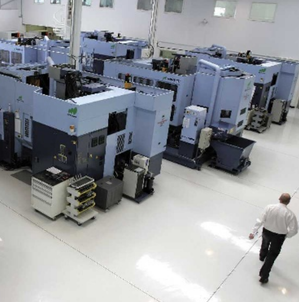
Above – seven Matsuura machines form the core of Honda Racing F1 Team's prismatic machining capability; Left – the company has also installed Mori Seiki mill-turn technology; Below – A hydraulic manifold machined on DMG technology by ING Renault F1 Team
