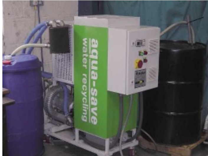
At Universal Engineering Company, concentrated oily waste, which typically represents less than 5 per cent of the original volume, is the only material that needs to be transported off site for safe disposal
