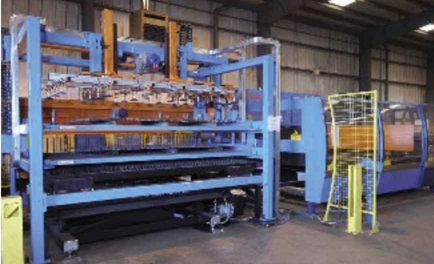
The new 4 kW Prima laser machine supports the company's drive in other ways. Its accuracy and repeatability allow many of Thompson's fabrication jigs and fixtures to be made in house
