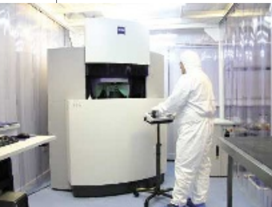
The Zeiss F25 is used by Kern in Germany to support its sub-contract operation. Uncertainty of measurement is 250 nm; resolution 0.25 nm
