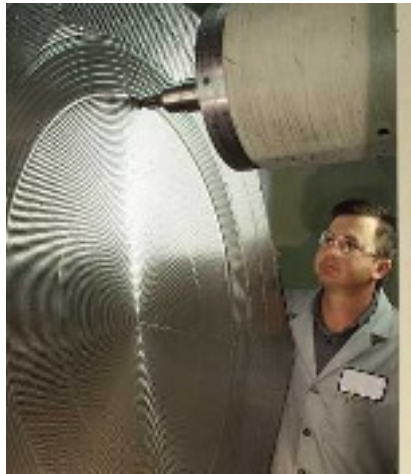
A Mitsui Seiki horizontal machining centre is to process 18 mirror segments, each 1.5 m across
