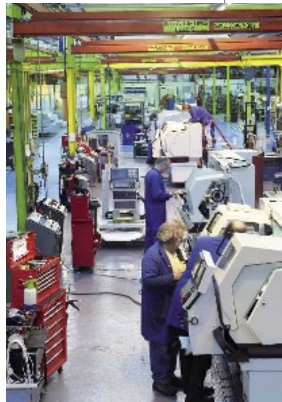
The flow-line has gone. Static build of the 600 Group's medium level CNC lathe technology, such as the Alpha (below), is the norm, as is assembly by multiskilled personnel
