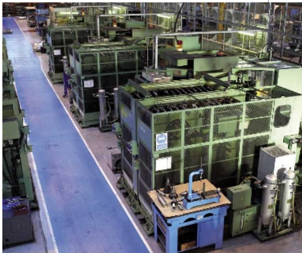
Moving to a make-to-order manufacturing environment has seen production on the company's Mitsui Seiki FMS retooled to support the delivery of machine sets of parts
