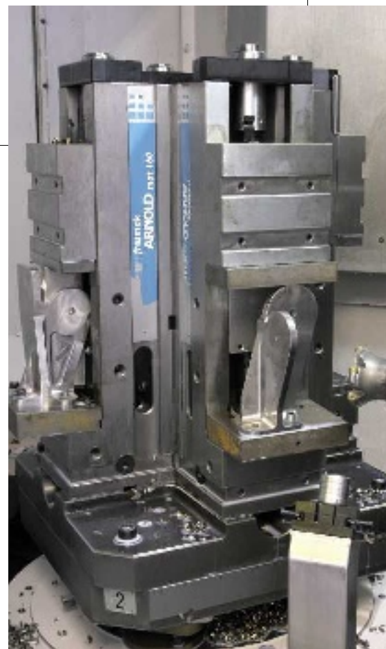
Prior to 2004, all of RD Precision's aerospace parts were machined on 3-axis vertical machining centres using multiple vice set-ups. The move to horizontal production has seen set-ups slashed and cycle times cut
