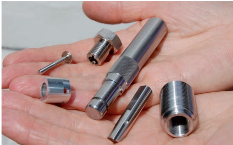
By investing in the multi-axis Citizen L20-VIII "I could scrap five cam autos. It's the best thing I've ever done," says Tony Mathews of Precision 82
