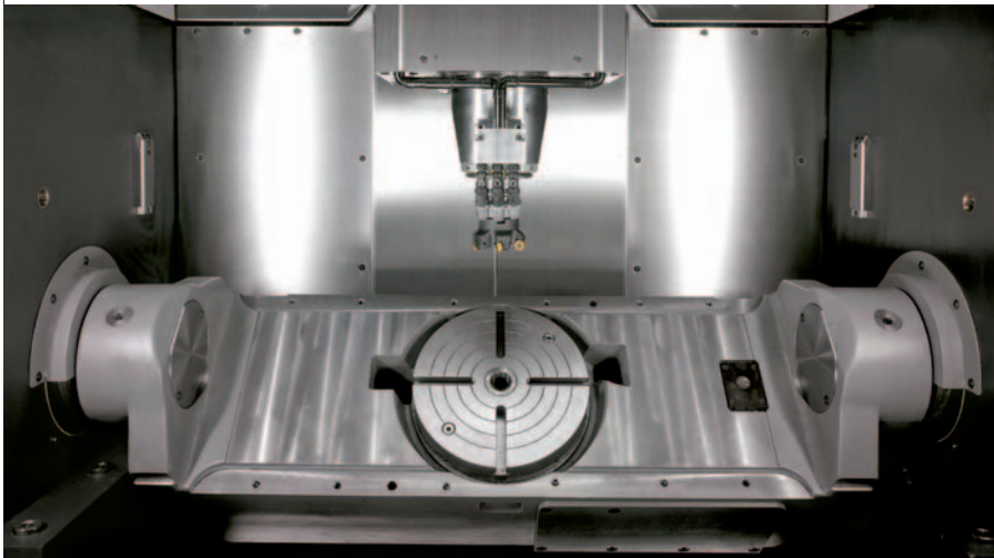
Hermle's B-300 unit is an entry-level 5-axis vertical machining centre for mould making and more
