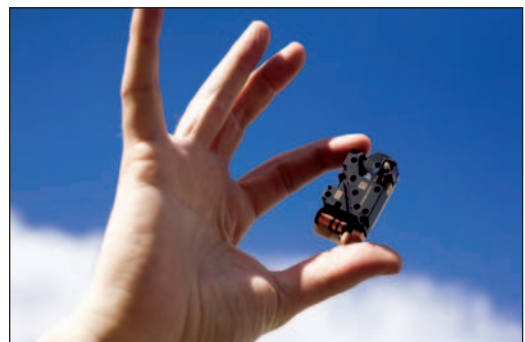
Above: DeepStream's 3d circuits are moulded inside robust plastic whilst the components mounted on the circuit are encapsulated.
