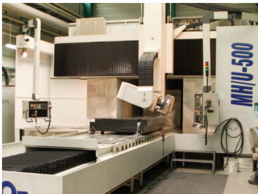
A recent investment, this machine can both grind and drill holes in Wenzel CMM granite tables
