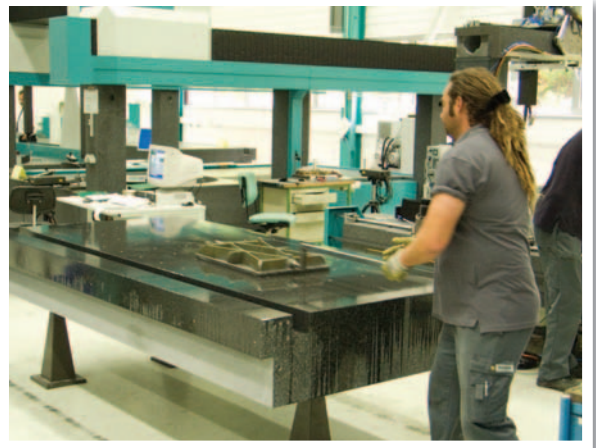
Hand lapping of a granite table. An established craft tradition within Wenzel and one that delivers precise flatness
