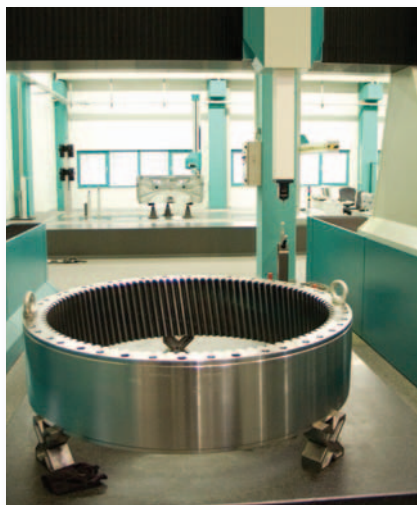
An LHF gantry type CMM shown here with a wind turbine gearbox component
