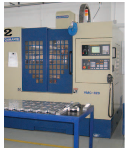
Hymec CNC Mauritius has opted for 12-off Matchmaker 800 VMCs. Already used by the company in the UK, it offers flexibility, while programs/set-ups can be proved in the UK
