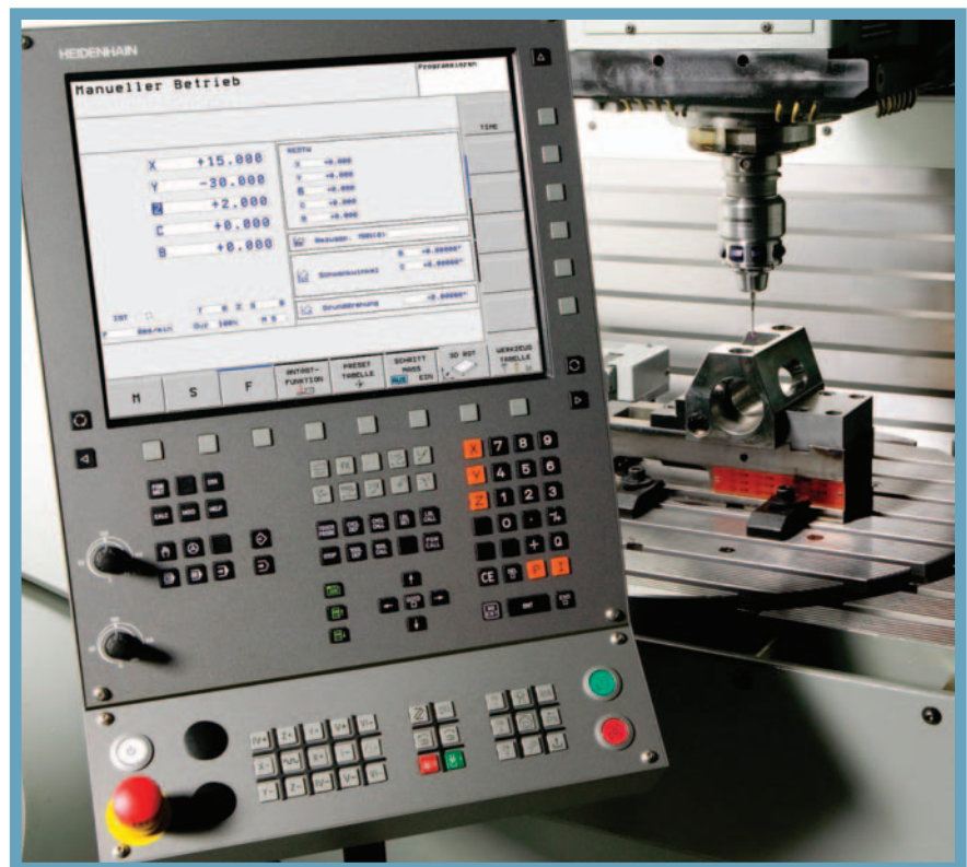
Heidenhain iTNC 530 is used by Winbro on machines that drill cooling holes in turbine components
