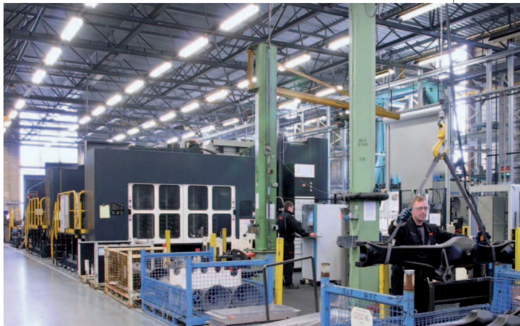
HPC Precision Engineering has added a Makino A100 twin-pallet machining centre to two similar machines in a flexible manufacturing system to boost its aerospace machining capacity
