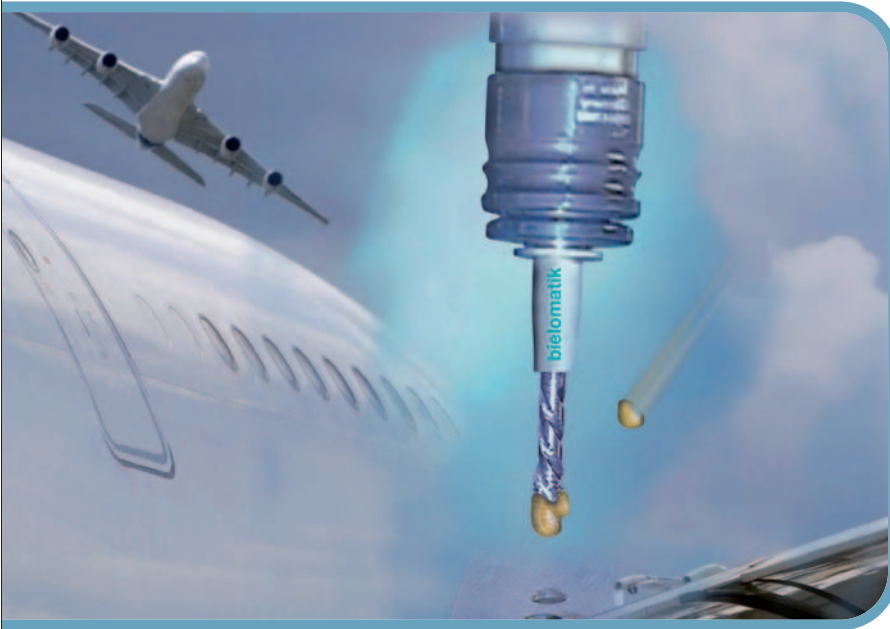
Cutting oil contamination at Airbus, Broughton threatened the company's investment in an automated drilling, countersinking and riveting process. Minimal quantity lubrication provided the answer
