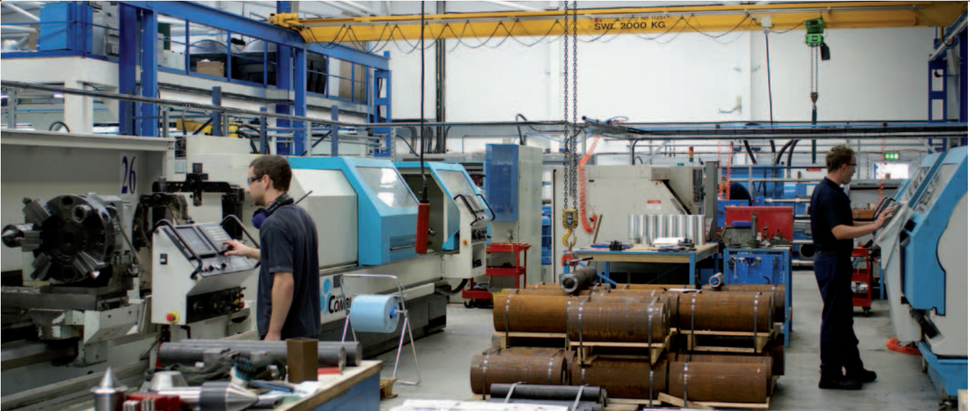
One of the suggestions from the workforce was to locate similar machines together, thus centralising shared tooling and workholding, for example
