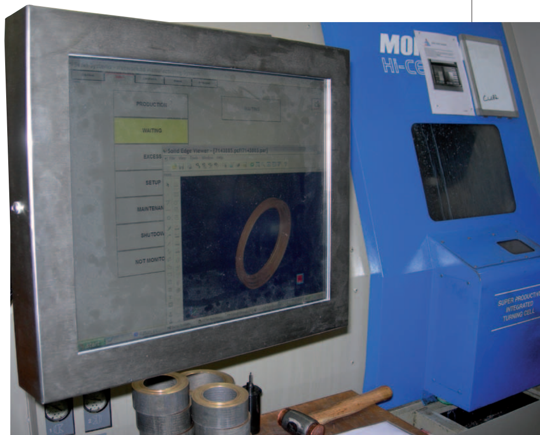
HMI's located adjacent to machine tools offer visibility of job-related information
