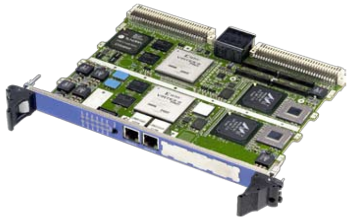
Figure 3: Curtiss-Wright VPF1, air-cooled version
