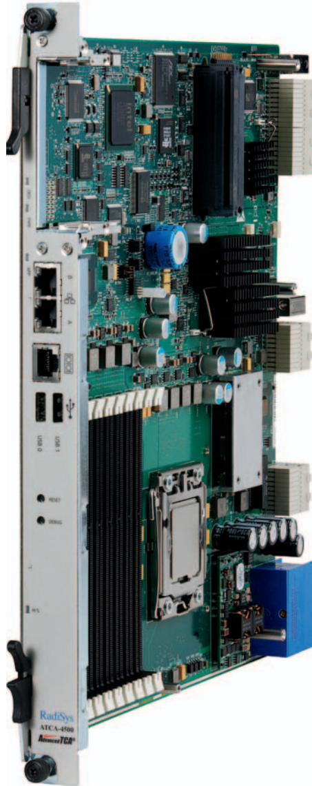
The ATCA-4500 is RadiSys' seventh generation single board computer. Based on the Intel Xeon processor, the single slot ATCA module is suitable for control plane and server functions in LTE wireless infrastructure, deep packet inspection, IPTV and IP multimedia subsystems.
