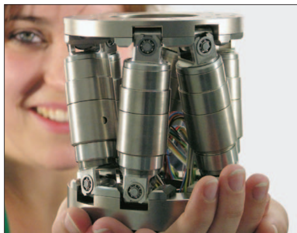
PI will be showing its miniature six axis positioning robot, appropriate for micro manipulation tasks
