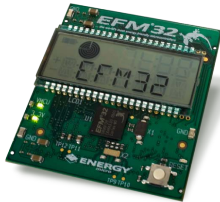
Figure 7: EFM32 directly driving a 160 segment LCD display
