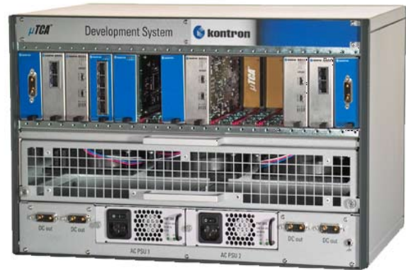
Figure 5 – MicroTCA sub-rack holding AdvancedMCs and power modules
