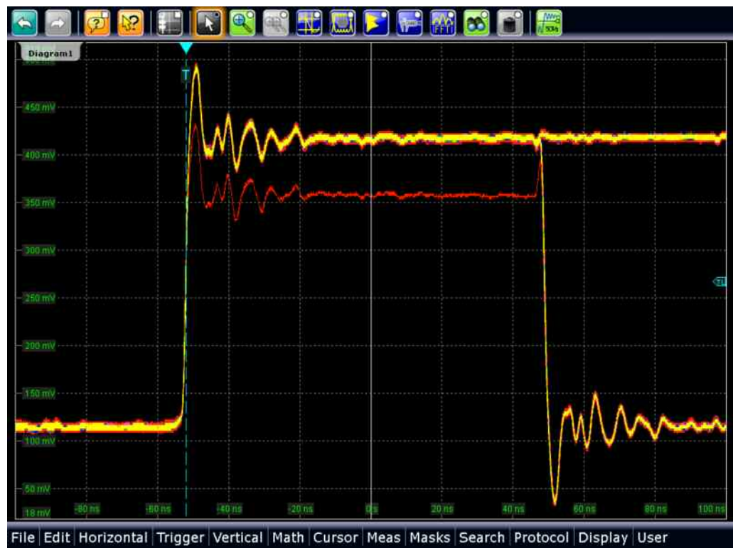
Figure 4: With the persistence view rare signal behaviors are highlighted. In this example sometimes a runt occurred.
