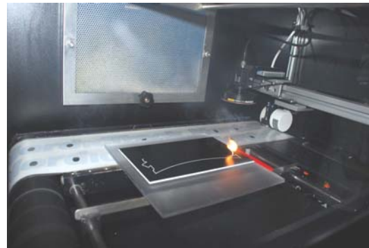
Figure 2: Laser Cutter Machine cutting a label
