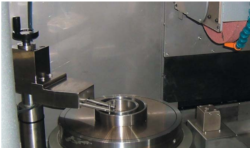
Okamoto's UPR-3NC combines variable hydrostatic slideway and air bearing technologies
