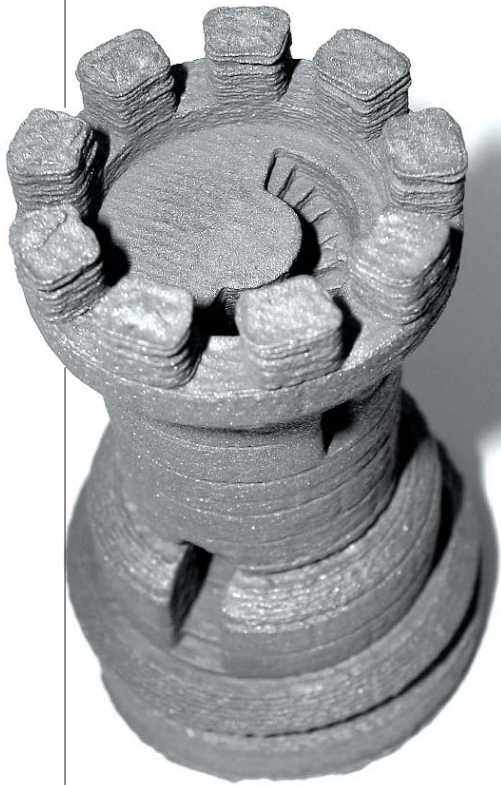
This chess piece was fabricated via Arcam's electron beam-based process
