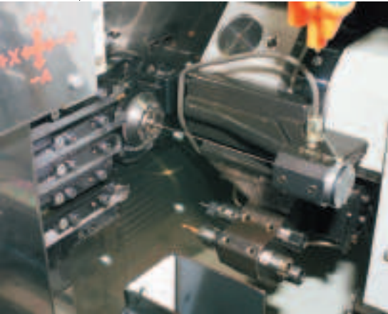
Integra Neuro Sciences is employing a number of tooling solutions on its Star sliding-head lathe, including this Botek gun drill supplied by Mollart
