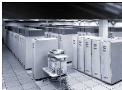
In 1996, ASCI Red was the first computer to benchmark at a teraflops. The system used around 10,000 Pentium Pro processors running at 200MHz and consumed 500kW of power plus an additional 500kW just to cool the room that housed it. Now, Intel has integrated similar computing power on one piece of silicon drawing just 62W.
