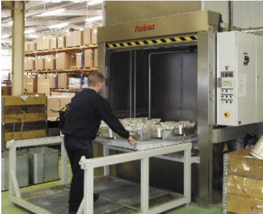
Catering equipment manufacturer IMC has switched from solvent to aqueous cleaning
