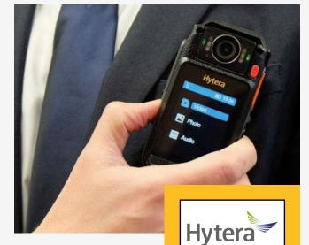
lens, I 6-megapixel image sensor and six infrared LED lights for filming in low-light conditions. It features one-touch operation for video capture, voice recording and emergency call.
