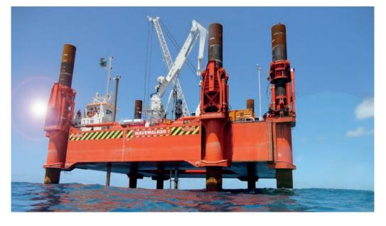
conditions, the jackup is also able to walk to areas of safe haven without the requirement for the use of tugs and similar support vessels in the event of deteriorating weather.
