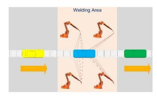
At the same time ATS Bus collects the running time and downtime of the machines carrying out the welding. This will be used to calculate the OEE later.
