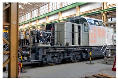
Here, at the site of the ALSTOM Locomotives Service - which is a joint enterprise with the Deutsche Bahn AG – the concept of the combined drive concept took concrete shape already in 2006. In that year, the ALSTOM engineers brought the first operable prototype of the hybrid shunting locomotive onto the rails. It was constructed on the chassis frame of the proven V100 locomotive with its two bogies. In addition to the
