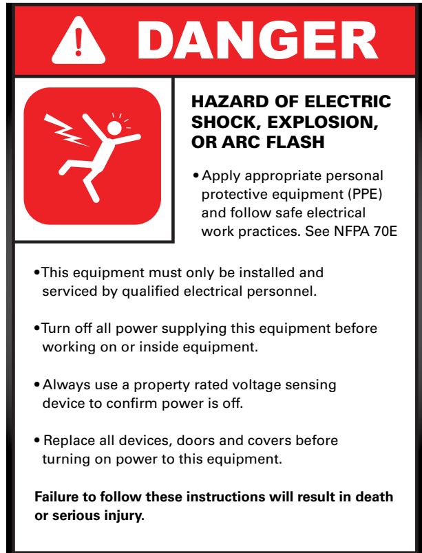
Figure 1. Example “Danger” label meeting NEC requirements.
