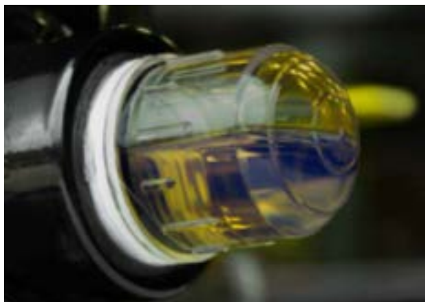
Figure 2. Replacing a flat sight glass with a 3D sight glass is a simple inexpensive modification that can greatly enhance the reliability of oil level checks.
