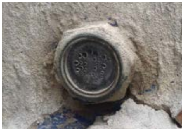
Figure 2. Replacing a flat sight glass with a 3D sight glass is a simple inexpensive modification that can greatly enhance the reliability of oil level checks.
