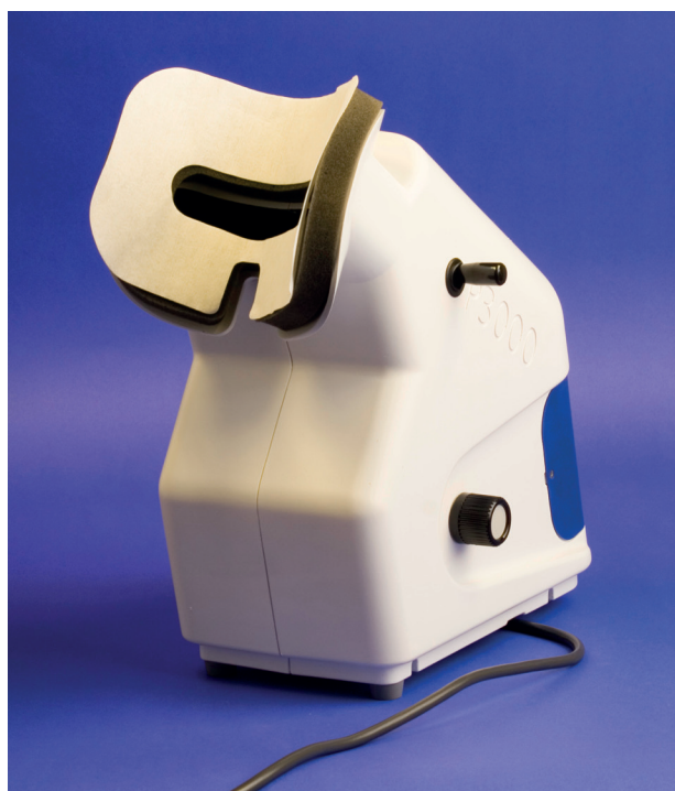
FIGURE 9 The Procyon P3000 pupillometer (image courtesy of Haag Streit UK)
